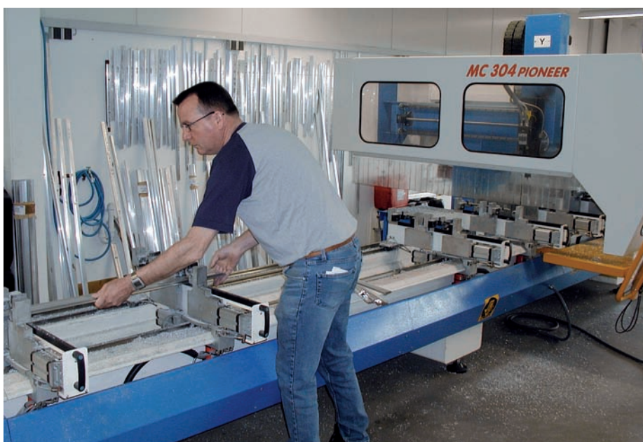
A modern CNC machine processes aluminium bars. Several hundred thousand bars are drilled and milled to the same standard of quality every year.
